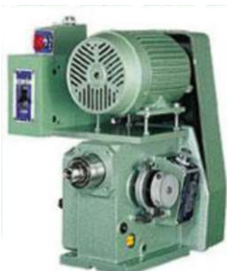
JT-6516A (Horizontal) Diameter of thread \phi 5-\phi 16
